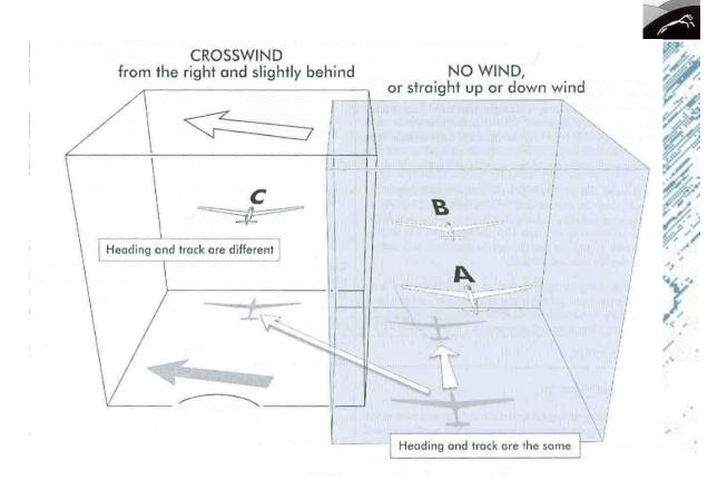
Where there is any kind of wind the air mass moves over the ground, carrying the glider (and its flight path) with it. If the glider in the previous slide maintains the same heading as it did when there was no wind, then any cross wind component in relation to that will carry the glider 'sideways' over the ground, and the track and heading will differ.
